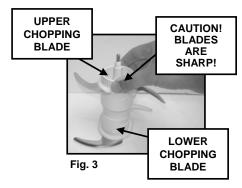
After having assembled the chopping blades, carefully place the chopping blade assembly onto the shaft of the food processor bowl.
